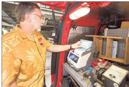
Les Moyer, co-owner of Admirals Lock and Safe, inputs key codes into a machine that can cut new car keys.
