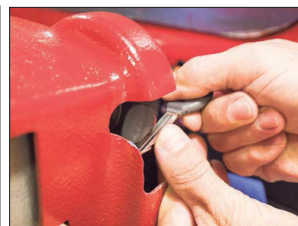
A sanding wheel removes the 'burrs' from a freshly-cut car key in the back of Moyer's work van.
